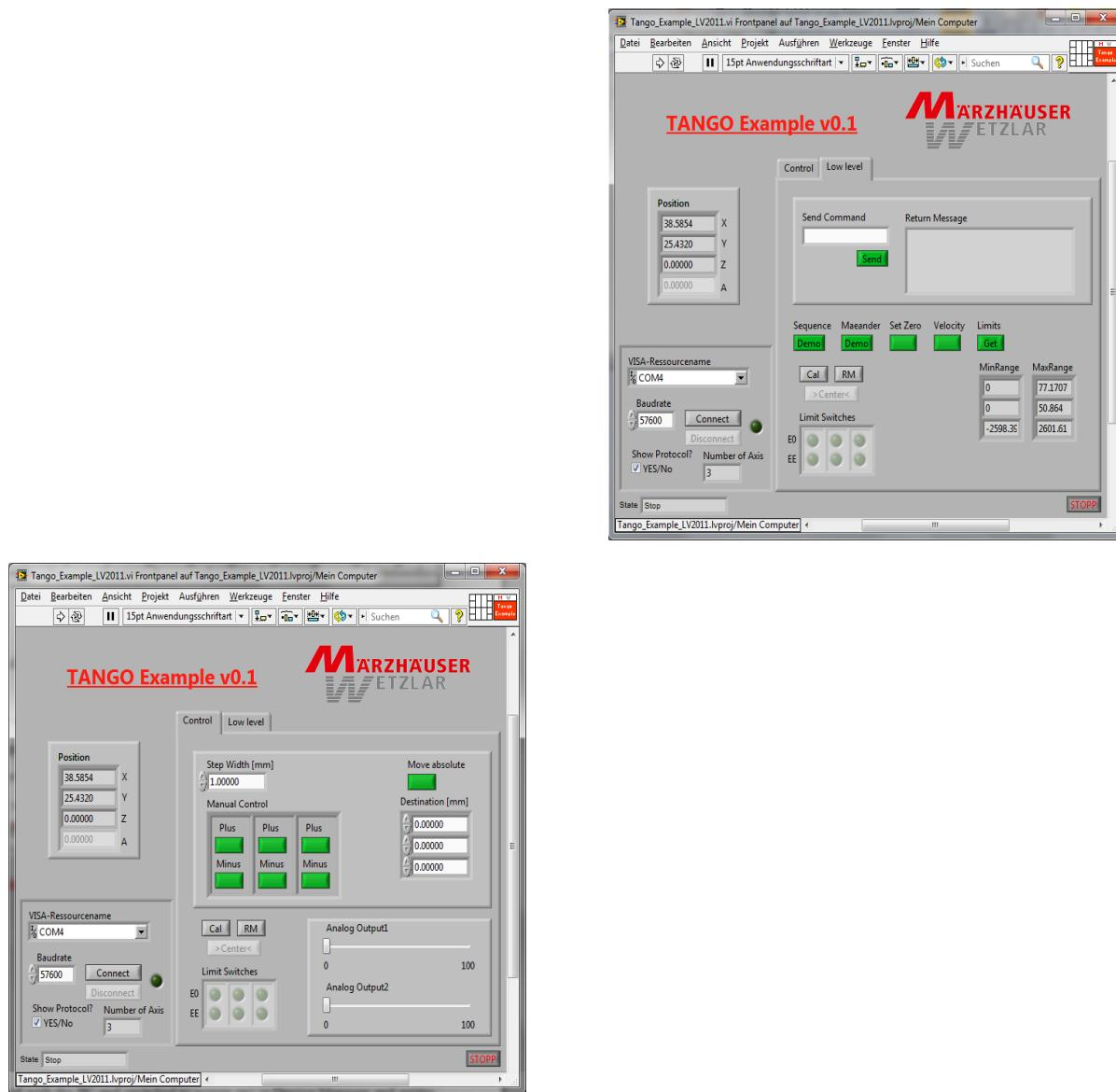
This example VI looks for a TANGO (connected with the PC and switched to power on) in Device Manager and writes the corresponding COM-Port in VISA-Ressourcenname as a pre-selection. The default baud-rate is 57600. After selecting the correct COM-Port the user is able to connect to TANGO.
