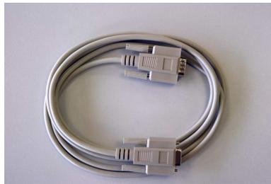
Fig. 1.3: RS232C Cable (2 m)
