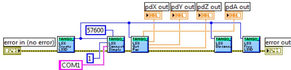
This example creates a TANGO-ID number to select the TANGO, which is addressed for the command. A connection to the TANGO is established with virtual COM-Port 1 and Baud-Rate 57600. The actual position of all axes is read out and the TANGO is disconnected. Last step is to free the created TANGO-ID number.
