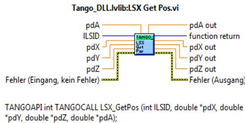
In all such "Get" VIs just connect only required output parameters. It is useless to connect input parameters because they will be ignored anyway and won't have any effect.
