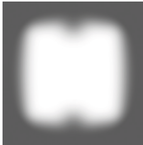
Distance LED module - lens too large
