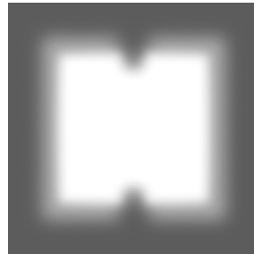
Distance LED module - lens too small
